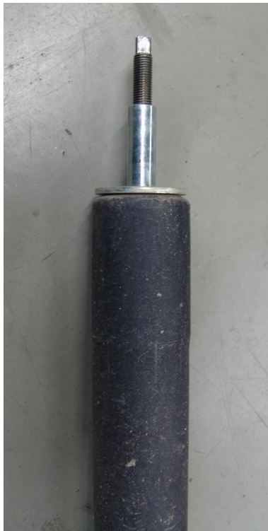
Preparation of the damper - extension of the rebound travel (Series condition)
